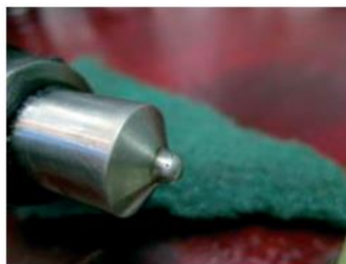
Nozzle condition before cleaning & after cleaning with a nylon sponge.
