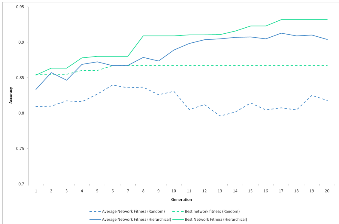
Figure 21: Average and best network accuracy for the population during the architecture search for the Fashion-MNIST problem.
