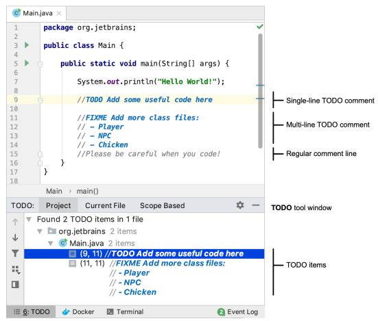
Figure 3. IntelliJ TODO Tool Window
