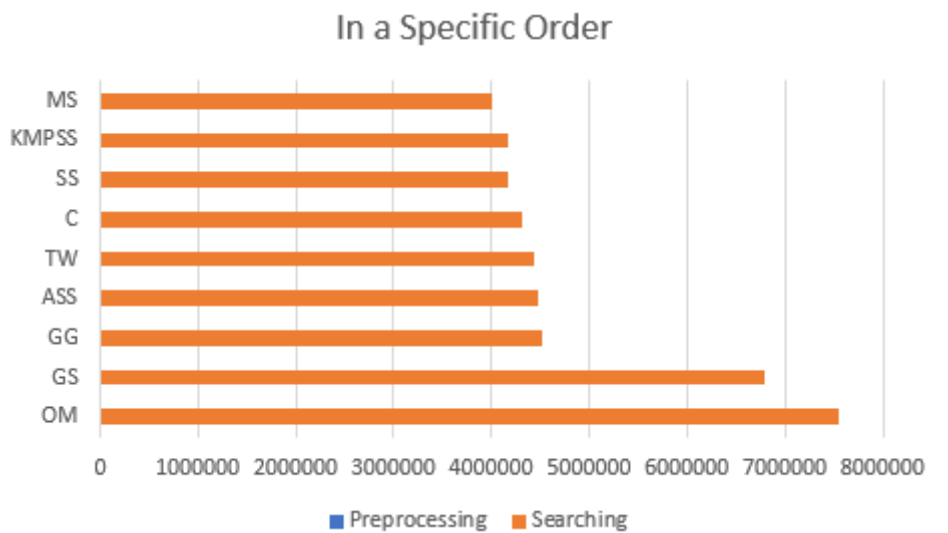
Figure 130: Searching the first occurrence of small patterns by comparing in a specific order.
